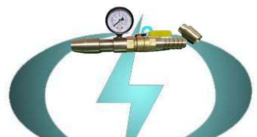
The test is made by spraying the enclosure from all practicable directions with a jet of water from the Premiers IP X5/6 test nozzle as shown in figure 6 of IEC 60529. This device is used for the verification test of the degree of protection to the risks of water penetration provided by wrapper of equipment in compliance with the second digit No. 5 (IPX5) and the second digit No. 6 (IPX6) according to IEC 60529.
