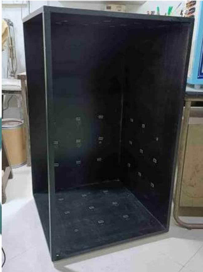
Dull black-painted plywood approximately 20 mm thick is used for the test corner.
